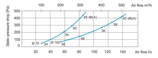
The static pressure drop is measured in accordance with ISO standard 5167-1. The noise level is measured according to ISO standard 3741.
